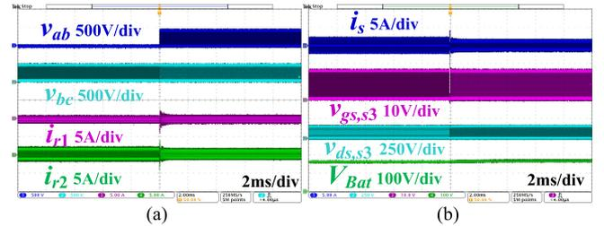
Fig. 25. Transition from Mode 2-C to Mode 3-C,  $V_{dc-link} = 420$  V and  $I_{Bat} = 1$  A. (a) H5-bridge waveforms. (b) Battery-side full-bridge waveforms.
