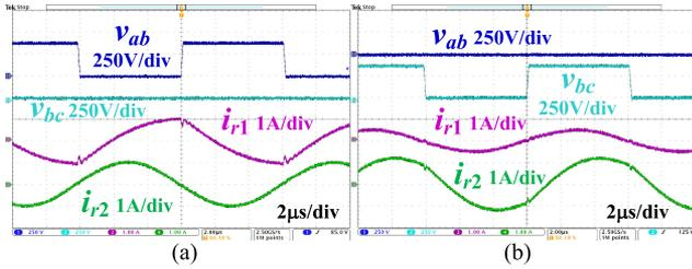
Fig. 15. Steady-state waveforms in (a) Mode 1-C with  $V_{dc-link} = 380$  V and  $I_{Bat} = 1$  A and (b) Mode 2-C with  $V_{dc-link} = 360$  V and  $I_{Bat} = 1$  A.
