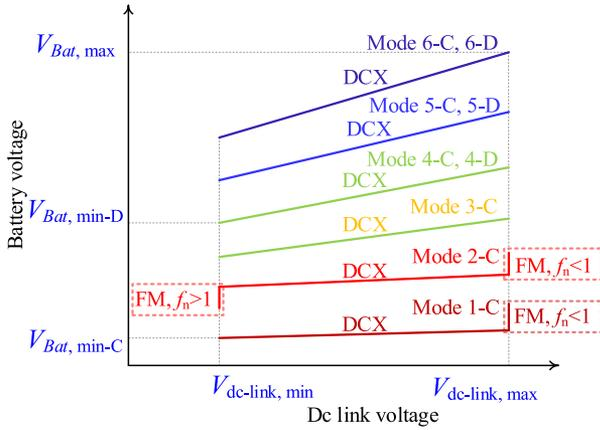
Fig. 9. Voltage range mapping between the battery and the dc link.
