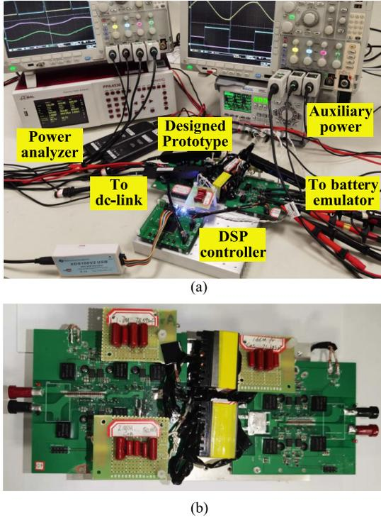
Fig. 14. (a) Experimental setup. (b) Designed prototype.
