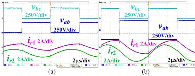
Fig. 16. Steady-state waveforms in (a) Mode 3-C with  $V_{dc-link} = 400$  V and  $I_{Bat} = 1$  A and (b) Mode 4-C with  $V_{dc-link} = 360$  V and  $I_{Bat} = 2.6$  A.
