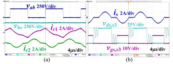
Fig. 18. Steady-state waveforms in Mode 1-C,  $f_s < f_r$ ,  $V_{dc-link} = 420$  V, and  $I_{Bat} = 1$  A. (a) H5-bridge waveforms. (b) Battery-side full-bridge waveforms.
