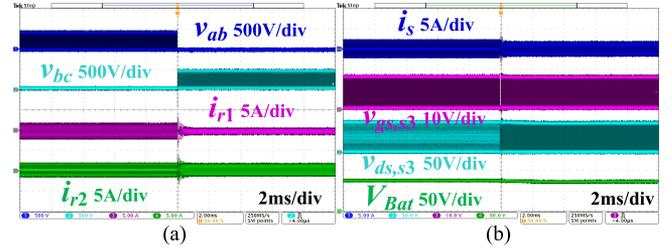
Fig. 24. Transition from Mode 1-C to Mode 2-C,  $V_{dc-link} = 420$  V and  $I_{Bat} = 1$  A. (a) H5-bridge waveforms. (b) Battery-side full-bridge waveforms.
