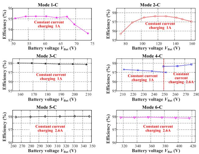
Fig. 29. Measured efficiency in the CC charging state.
