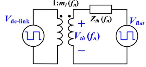
Fig. 5. Unified circuit model to describe six modes.
