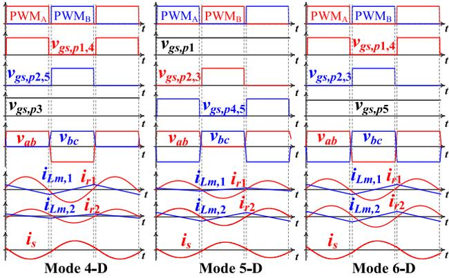
Fig. 3. Gate signals,  $v_{ab}$ ,  $v_{bc}$ , and resonant current waveforms in the proposed reconfigurable DCX in the discharging process (Modes 4-D–6-D).
