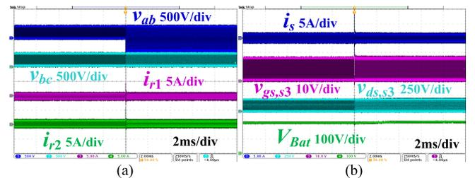
Fig. 26. Transition from Mode 3-C to Mode 4-C,  $V_{dc-link} = 420$  V and  $I_{Bat} = 1$  A. (a) H5-bridge waveforms. (b) Battery-side full-bridge waveforms.
