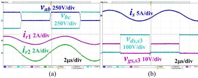
Fig. 22. Steady-state waveforms in Mode 5-D,  $V_{dc-link} = 327$  V and  $I_{Bat} = 2.52$  A. (a) H5-bridge waveforms. (b) Battery-side full-bridge waveforms.
