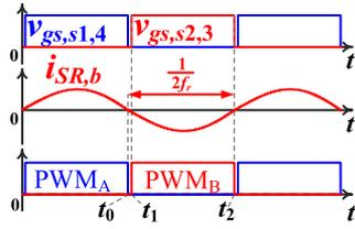
Fig. 8. SR waveforms  $f_s = f_r$  in the discharging process.
