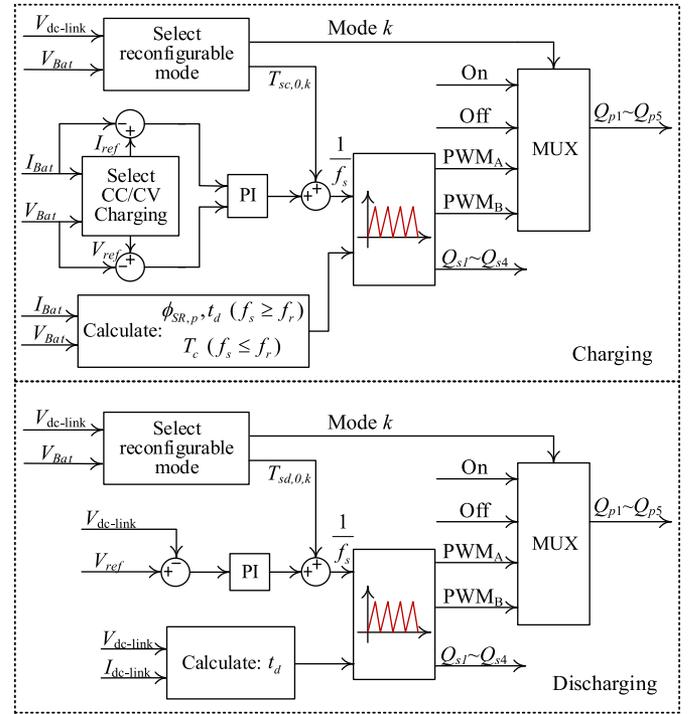
Fig. 13. Control diagrams in charging and discharging processes.
