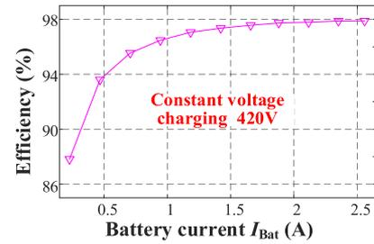
Fig. 30. Measured efficiency in the CV charging state in Mode 6-C.
