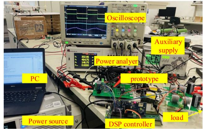
Fig. 11. Photograph of the laboratory test bench.
