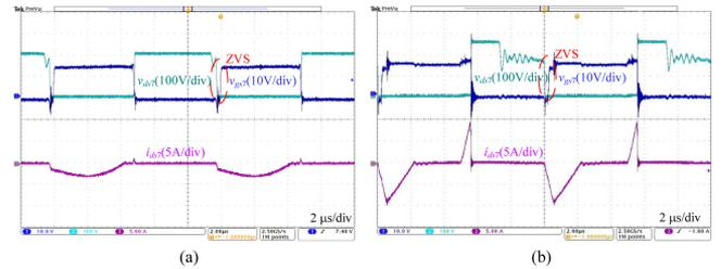
**Fig. 16.** Soft-switching waveforms of the secondary-side MOSFET with RT1 operating in FB mode. (a)  $V_1 = 200$  V,  $I_1 = 2$  A. (b)  $V_1 = 250$  V,  $I_1 = 2$  A.
