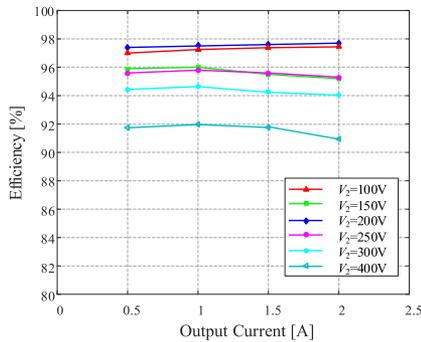
Fig. 19. Measured efficiency versus  $I_2$  with different  $V_2$  ( $V_1 = 200$  V,  $I_1 = 2$  A).
