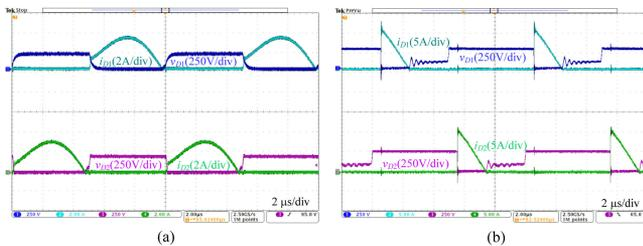
**Fig. 14.** Waveforms of diode voltages and currents when RT1 operates in FB mode with  $I_1 = 2$  A. (a)  $V_1 = 200$  V. (b)  $V_1 = 250$  V.
