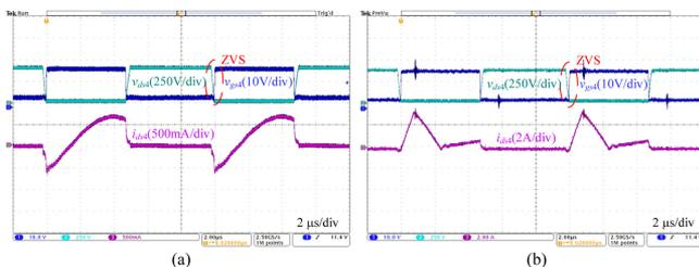
**Fig. 15.** Soft-switching waveforms of the primary-side MOSFET in HBID mode. (a)  $V_1 = 100$  V,  $P_1 = 50$  W. (b)  $V_1 = 200$  V,  $P_1 = 400$  W.
