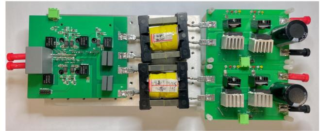
Fig. 12. Photograph of the designed SIDO LLC converter.
