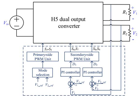
Fig. 10. Diagram of the digital control scheme.
