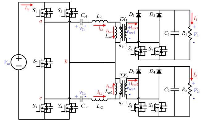
Fig. 1. Schematic of the proposed SIDO *LLC* topology.
