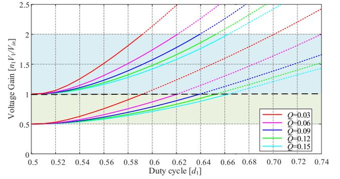
Fig. 6. Voltage gain curves versus  $d_1$  under different  $Q$ .
