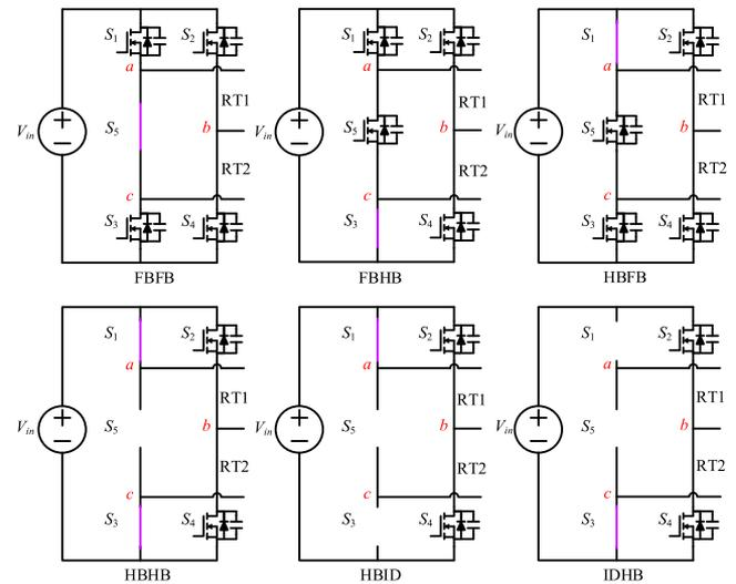
Fig. 2. Configurations of the H5 bridge.
