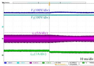
Fig. 18. Dynamic waveforms of load step down from 250 to 150 W.
