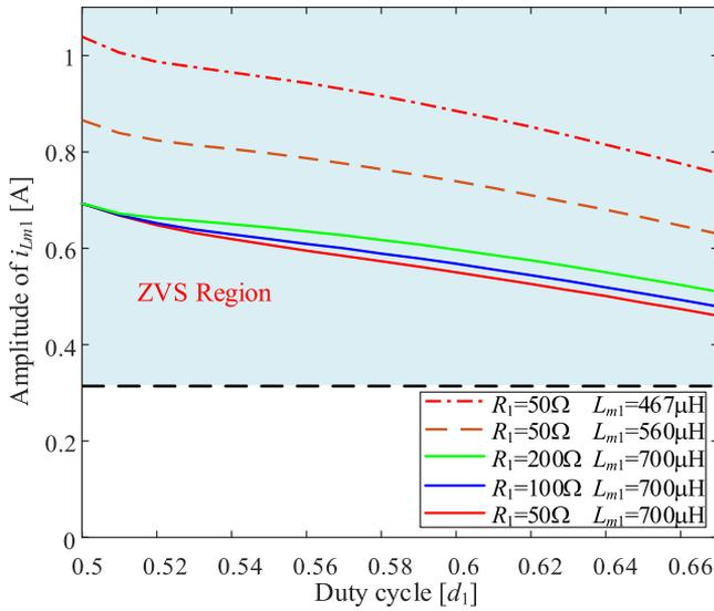
Fig. 8. Profiles of  $i_{L_{m1}}$  versus duty cycle with different  $R_1$  and  $L_{m1}$  when  $L_{r1} = 46.9\mu\text{H}$  and  $C_{r1} = 54\text{nF}$ .
