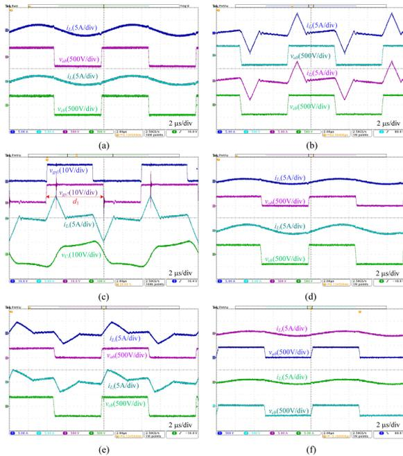
**Fig. 13.** Experimental steady state waveforms in different modes. (a) FBFB mode  $V_1 = V_2 = 200$  V,  $P_1 = P_2 = 400$  W. (b) FBFB mode  $V_1 = V_2 = 400$  V,  $P_1 = P_2 = 800$  W. (c) FBFB mode  $V_1 = 400$  V,  $P_1 = 800$  W. (d) HBFB mode  $V_1 = 100$  V,  $P_1 = 100$  W,  $V_2 = 200$  V,  $P_2 = 400$  W. (e) HBFB mode  $V_1 = 150$  V,  $P_1 = 300$  W,  $V_2 = 250$  V,  $P_2 = 500$  W. (f) HBFB mode  $V_1 = V_2 = 100$  V,  $P_1 = P_2 = 100$  W.
