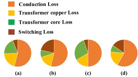
Fig. 9. Loss breakdown in different output voltages at heavy load condition.
