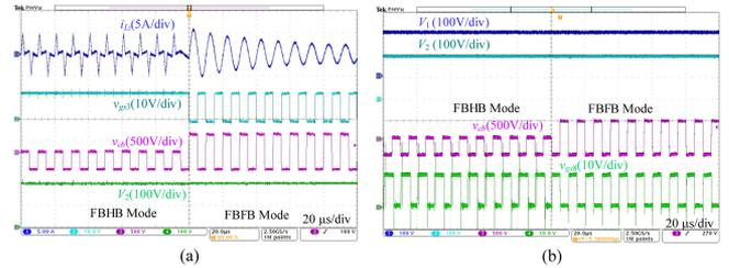
**Fig. 17.** Dynamic transition from FBHB Mode to FBFB Mode with  $V_1 = V_2 = 200$  V,  $P_1 = P_2 = 200$  W.
