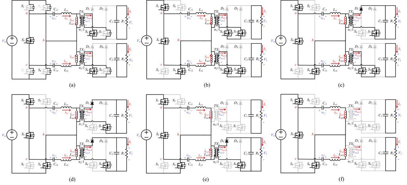
**Fig. 4.** Equivalent circuits over half switching cycle. (a) Stage I,  $t_0 < t \leq t_1$ . (b) Stage II,  $t_1 < t \leq t_2$ . (c) Stage III,  $t_2 < t \leq t_3$ . (d) Stage IV,  $t_3 < t \leq t_4$ . (e) Stage V,  $t_4 < t \leq t_5$ . (f) Stage VI,  $t_5 < t \leq t_6$ .
