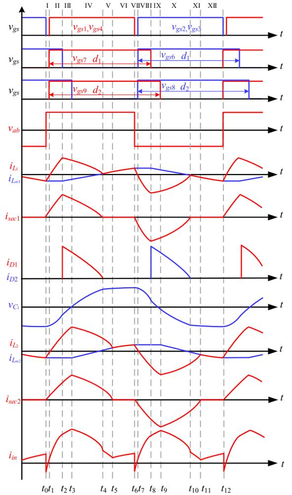
Fig. 3. Critical steady-state waveforms.
