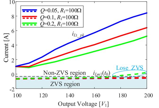
Fig. 7. Profiles of peak current and  $i_{L_{m1}}(t_0)$  versus output voltage under different  $Q$ .
