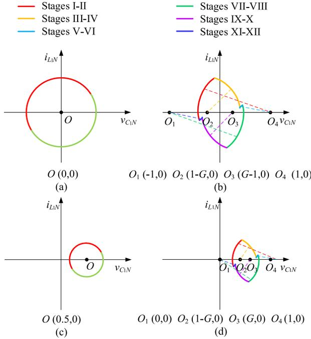
Fig. 5. Trajectory of RT1. (a) FB mode with 50% secondary-side duty cycle. (b) FB mode with more than 50% secondary-side duty cycle. (c) HB mode with 50% secondary-side duty cycle. (d) HB mode with more than 50% secondary-side duty cycle.
