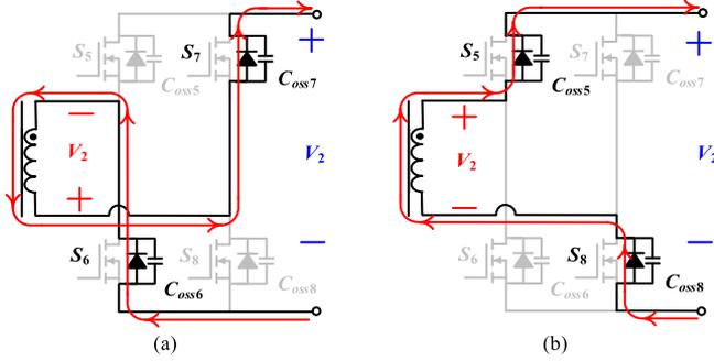
Fig. 8. Current path in the dead time before  $S_{6,7}$  are turned on in (a) ZVS condition, (b) non-ZVS condition.
