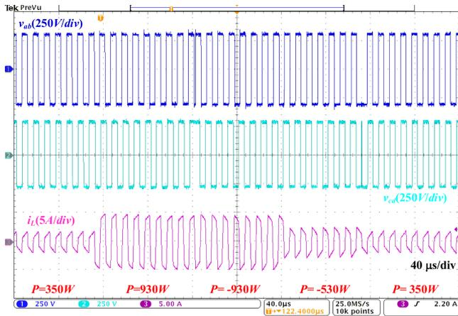
Fig. 17. Experimental waveforms with SPS modulation when the power flow direction changes.
