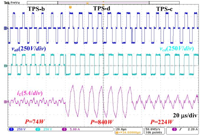
Fig. 19. Experimental waveforms in the forward mode with TPS when the load changes.
