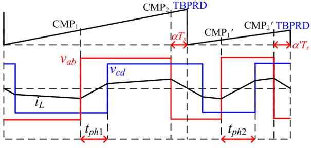
Fig. 5. Key waveforms of the ZCP based VFM modulation.
