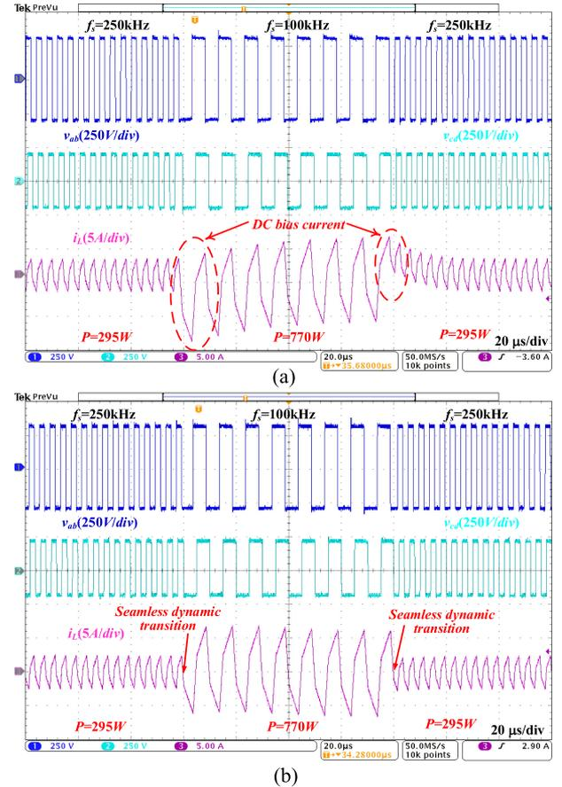
Fig. 16. Experimental waveforms in the forward mode with VFM modulation when load changes using (a) conventional method and (b) proposed method.
