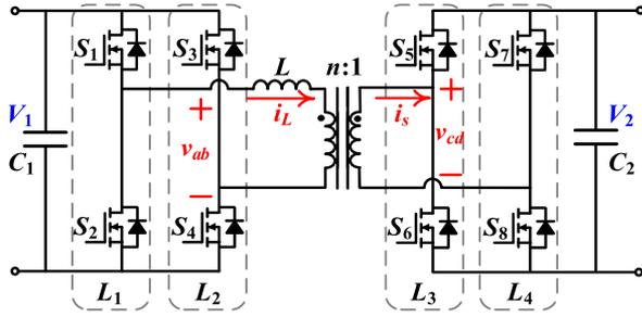
Fig. 1. Schematic of a typical DAB converter.
