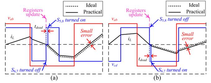
Fig. 9. Effect of dead time when the converter changes (a) from non-ZVS condition to ZVS condition, (b) from ZVS condition to non-ZVS condition, with SPS modulation.
