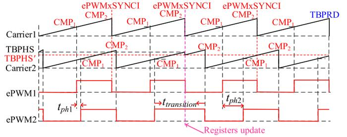
Fig. 2. Mechanism of switch pattern generation using the conventional method.
