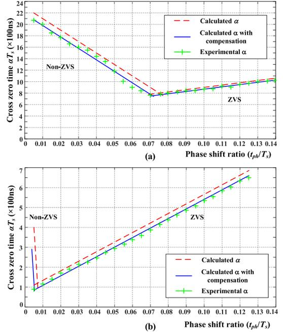
Fig. 14. Theoretical and experimental results of  $\alpha$  when (a)  $V_2 = 200$  V, and (b)  $V_2 = 280$  V.
