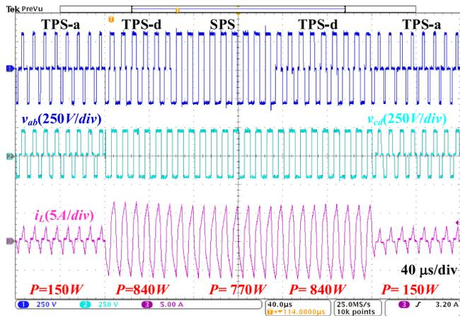
Fig. 18. Experimental waveforms in the forward mode when the modulation method changes.
