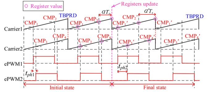
Fig. 7. Mechanism of switch pattern generation with the proposed method.
