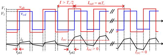
Fig. 3. Waveforms of DAB when the load current increases with the conventional SPS modulation.
