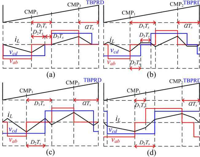
Fig. 6. Key waveforms of the four optimized modes with the ZCP based TPS modulation, (a) light load TPS-a, (b) light load TPS-b, (c) light load TPS-c, and (d) heavy load TPS-d.
