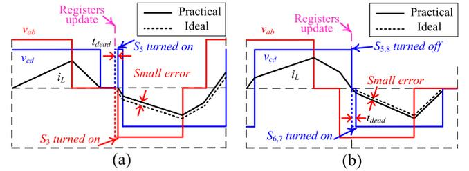
Fig. 10. Effect of the dead time when the converter changes (a) from non-ZVS condition to ZVS condition, (b) from ZVS condition to non-ZVS condition, with TPS modulation method.
