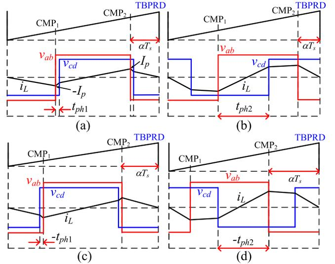
Fig. 4. Key waveforms of four modes in ZCP based SPS modulation, (a) non-ZVS in the forward direction, (b) ZVS in the forward direction, (c) non-ZVS in the backward direction, and (d) ZVS in the backward direction.
