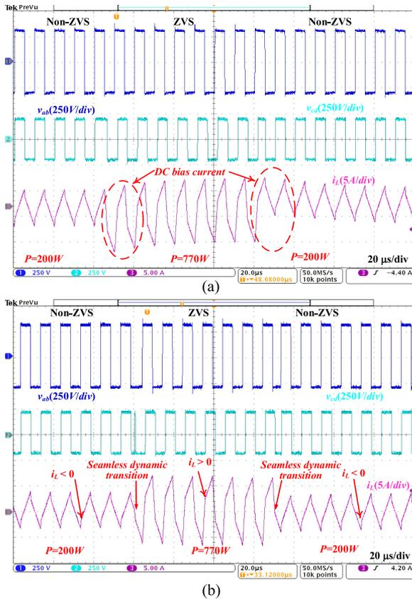
Fig. 15. Experimental waveforms with SPS modulation when the operation changes between non-ZVS region and ZVS region in the forward direction with (a) conventional method and (b) proposed method.
