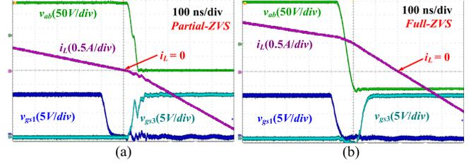
Fig. 13. Experimental waveforms of  $v_{ab}$  and  $i_L$  when (a) the current polarity reverse during the dead time and (b) the current polarity reverse after the dead time.
