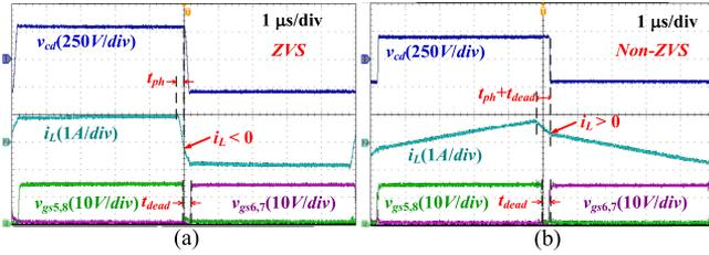
Fig. 12. Experimental waveforms of  $v_{cd}$  and  $i_L$  in (a) ZVS condition, (b) non-ZVS condition.
